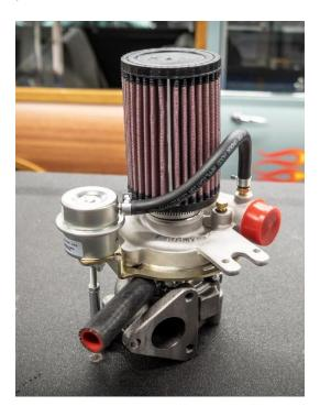
Apply high temp RTV to turbo oil drain fitting.
