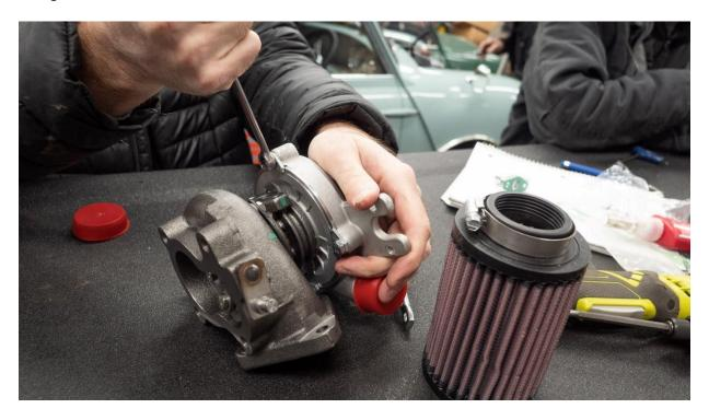
Clock compressor and turbine housings per photo. Note clocking of turbine inlet, compressor outlet and oil feed.
