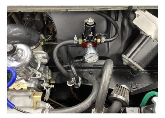
Install short hose from intake pipe fitting to this port on carburetor.
