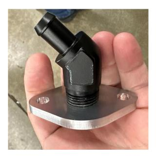
Use 5/16 UNC nuts to secture plate to clutch housing. Use high temp RTV to seal plate to clutch housing.
