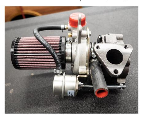
Install new waste-gate actuator hose (from bag 3.2) and secure with re-used hose clamps. Install air filter and secure with hose clamps.
