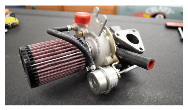
Install waste-gate actuator onto new bracket using existing hardware. Make sure you have a few pounds of tension to keep the waste-gate valve closed. This may be adjusted later to control max boost pressure.
