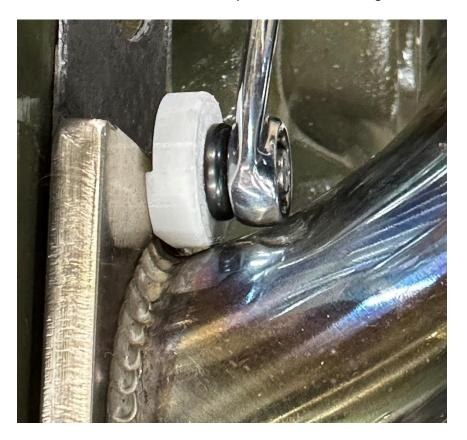
Torque manifold nuts to 15-21 Nm (11-15 Ft-lbs)
