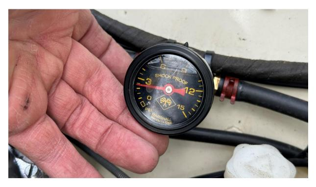
Adjust boost pressure. Keep boost pressure around 6-8 psi at beginning. 12 psi is max pressure allowed. We have safely taken engines to over 20 psi during testing.
