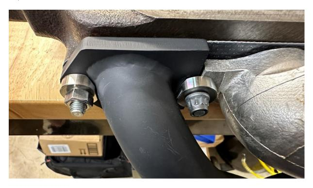
Use thin washers (4mm thick), if required, for tight spot of stud to header. Stepped washers may also be ground to fit these locations.
