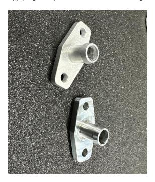
Install  $\frac{1}{2}$ ' high temp silicon hose to oil drain before installation of fitting. Install new nipple fitting using M6x16 hex screws and M6 washers. Torque to 6-9 Nm (4-7 Ft-lbs)
