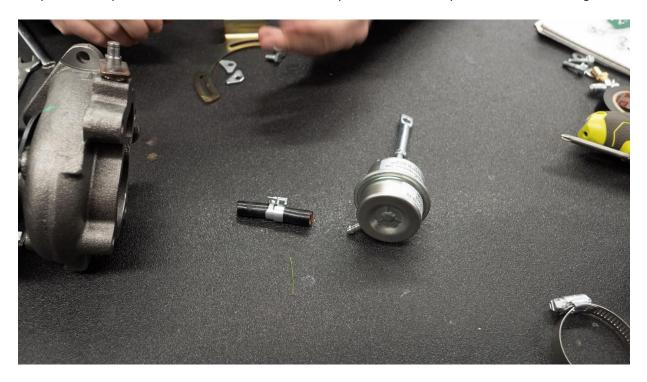
Remove inner nipple on turbo compressor and install new 1/8 NPT brass plug in its location
