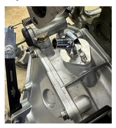
If you don't have a hole in the clutch housing, we recommend installing a drain fitting to the fuel pump mounting location. A kit for this will be available in the future.
