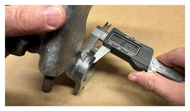
Select either 0mm, 1mm or 2mm stepped washers depending on difference in thickness of the manifold. These washers are located in bag 1.2. The mid washers have a relief machined into them for weld clearance on new turbo exhaust manifold.
