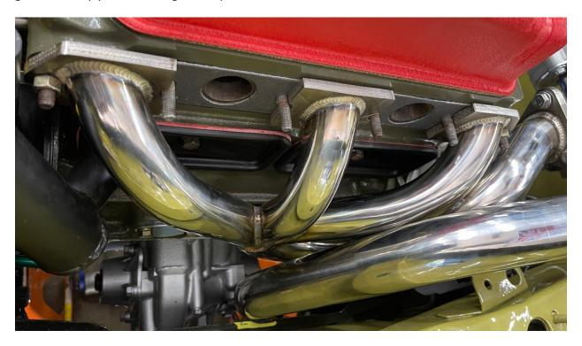
Install new exhaust/intake manifold gasket.
