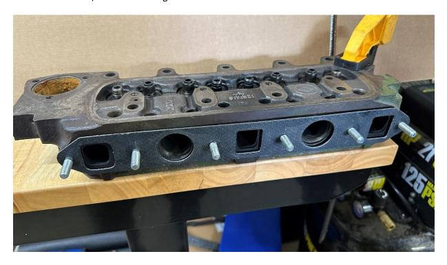
Select proper manifold washers by measuring the thickness of new exhaust header flange. Measure each hardware location that is located next to the intake manifold (4 locations)
