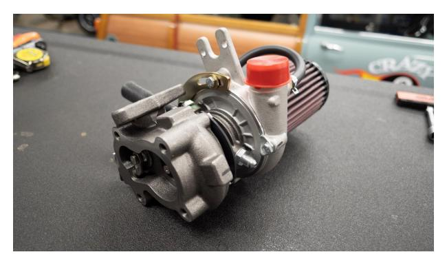
Install new waste-gate bracket from bag 3.1. Use existing M6 hardware and two M6 washers to mount new bracket to compressor housing. Install new waste gate hose from compressor outlet to wastegate.
