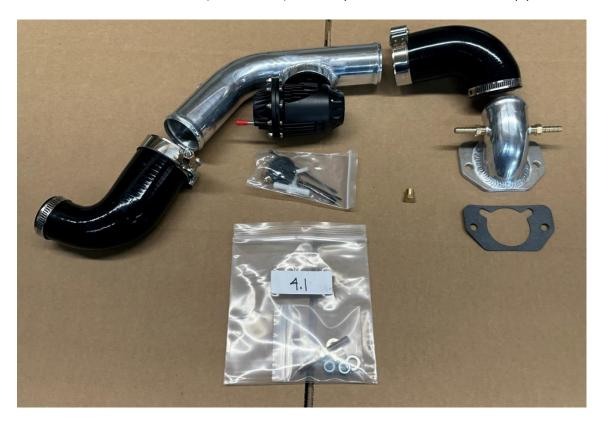
Install 1/8 NPT pipe plug from bag 4.1
