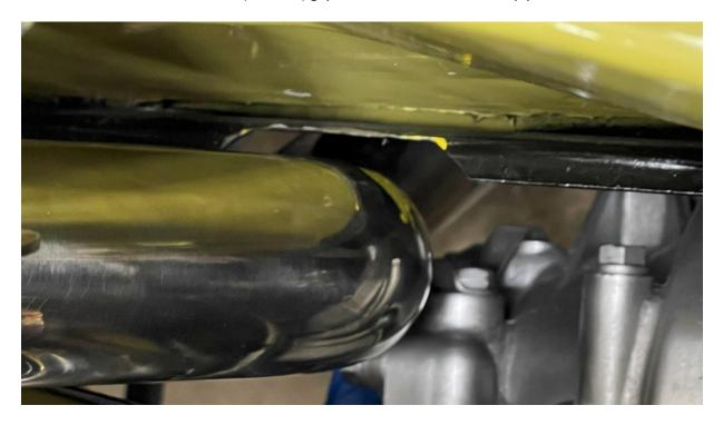
You may want to trim the end off the down pipe to improve installation. We have removed up to 50mm (2 inches) from the end of the downpipe to do this.
