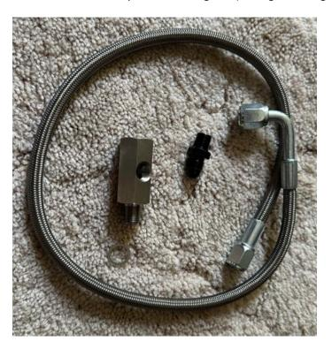
Remove oil pressure sender from engine. Install new 3-way T from bag 7.1. Install old pressure sender at end of T as shown (1/8 BSPT). Install AN4 to 1/8 NPT straight fitting to side of T. Attach oil feed hose as shown.
