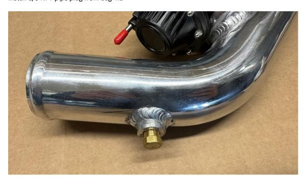
Install intake elbow onto carburetor and gasket onto carb flange from bag 4.1. Secure with 5/16 UNC hex head screws and M8 washers.
