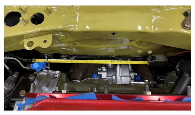
We recommend at least a 10mm (3/8 inch) gap between frame and down pipe.
