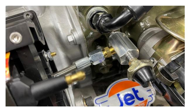
Connect 90 degree fitting to turbo inlet feed.
