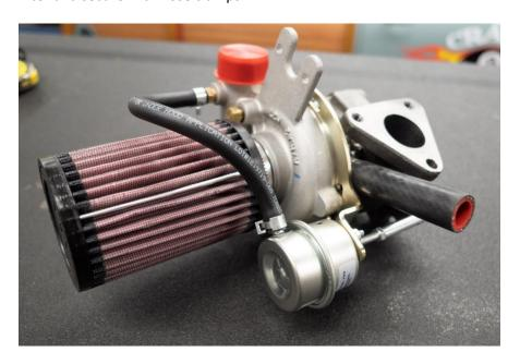
Install oil supply fitting with included sealing washer from bag 3.2. The turbo is ready for installation.
