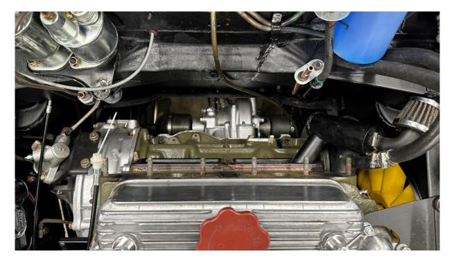
Replace studs if damaged or chase 5/16-24 exhaust studs with die nut if required.
