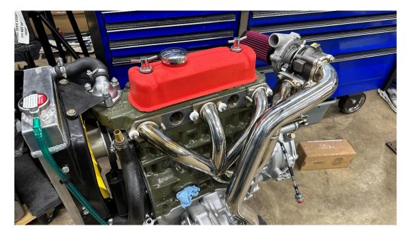
Sometimes the downpipe will need to be modified (dented) in order for the parts to fit correctly. We want the header and downpipe to slightly interfere so they don't rattle. We recommend only modifying the downpipe not the header.
